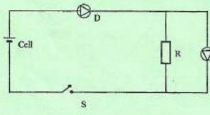
When the cell terminals are reversed and the switch is closed, the voltmeter reading is zero.
