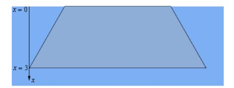
Note that we started the *x*-axis at the surface of the water and by doing this *x* will give the depth of any point on the plate below the surface of the water. This in turn means that the bottom of the plate will be defined by x = 3.
