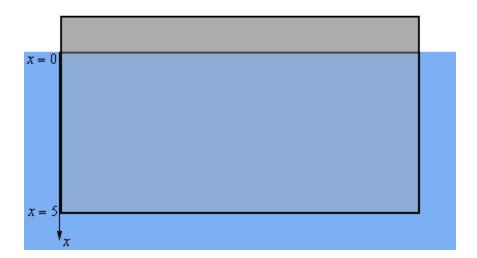
Note that we started the *x*-axis at the surface of the water and by doing this *x* will give the depth of any point on the plate below the surface of the water. This in turn means that the bottom of the plate will be defined by x = 5.
